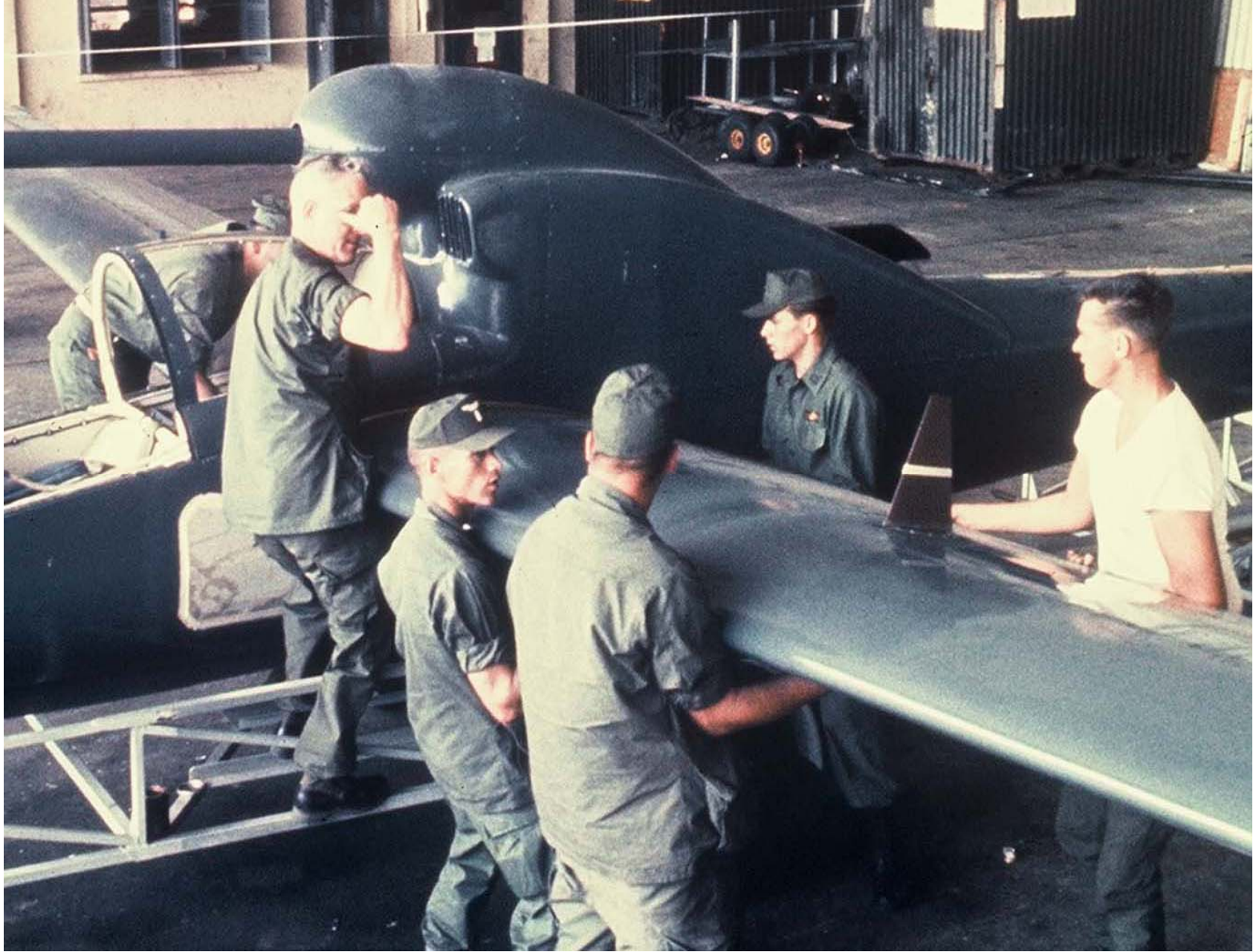
Crew Installing Port Wing
